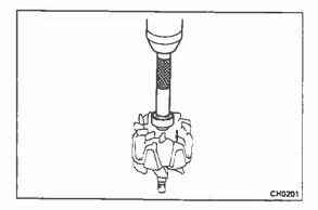
(b) Using SST, install the rear bearing and bearing cover onto the rotor shaft.
