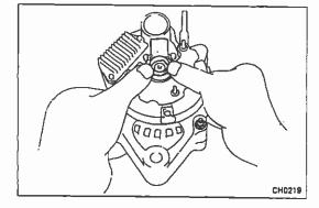
(d) Install the brush holder cover to the rear end frame.
